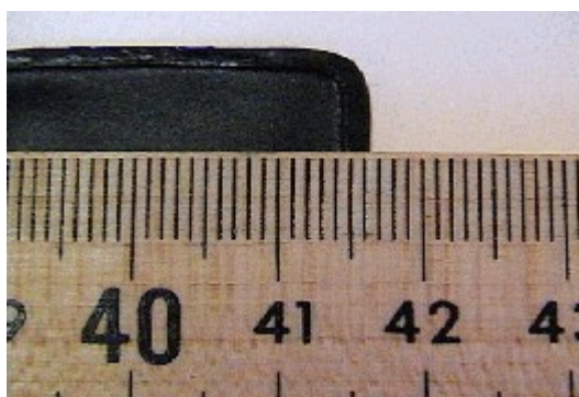
Figure 2. An example of a meter sticks reading. The object's length is measured to be 41.64 cm. (See text for description.)
