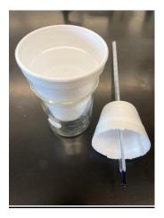
The calorimeter used in this experiment is made by two white Styrofoam coffee cups. The bottom of the top-cutoff Styrofoam coffee cup is pierced in order to insert a thermometer. For added stability, students may place the Styrofoam coffee cup into a 250-mL breaker.
