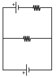
Three-branched circuits have three branches joining the two junction points. They also have three loops, which I call the top loop, the bottom loop and the outside loop.
