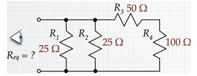
a) 40.29  $\Omega$ . b) 0.829  $\Omega$ . c) 11.5  $\Omega$ . d) 91.17  $\Omega$ . e) 141.54  $\Omega$ . R1 and R2 are parallel with each other, and with R3+R4.  $\frac{1}{R_{eq}} = \frac{1}{R_{1}} + \frac{1}{R_{1}} + \frac{1}{R_{3+4}} \rightarrow 1/25 + 1/25 + 1/150 = 13/150 \rightarrow 1/13/150 = 11.5$
