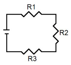
In a series circuit, a wire will carry current into one resistor, then into the next, and so on, passing through all of the resistors one at a time. Charges moving through a series circuit pass through all of the resistors of the circuit.
