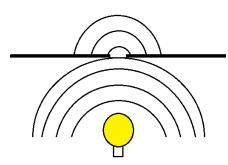
When waves pass an obstacle, they will bend around the corners and spread (propagate) out into the surrounding area. The waves treat the object they are diffracting around as if it were a source of the waves.
