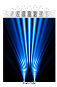
The double slit experiment involves shining a single light source toward two slits, and observing the resulting constructive and destructive interference caused by the refraction.
