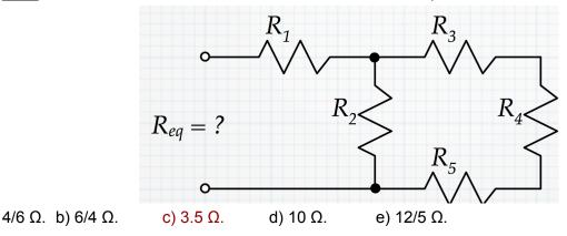
R3/4/5 are in series with each other and parallel to R2, R1 is series with those two. R1+1/(1/R2 + 1/(R3+4+5)  $\rightarrow$  2+1/( $\frac{1}{2}$ +  $\frac{1}{6}$ )  $\rightarrow$  2+6/4 = 3.5
