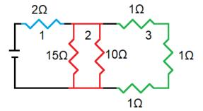
Section 1 is in series with section 2. The resistors in section 2 are in parallel with each other, and with section 3. The resistors in section 3 are in series, and form a parallel connection with section 2
