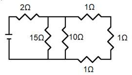
First, start by identifying which areas are in series and which are in parallel
