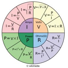
This diagram is a tool that shows all of the formulas for calculating current, voltage, resistance, and power.
