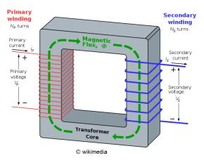
To change the voltage, we make use of transformers. Transformers use two coils of wire wrapped around sections of a circular piece of iron. As electricity passes through one set of coils, it creates a magnetic field that passes through the iron. As this magnetic field passes through the coils on the other side, the moving magnetic field will create an electrical current in these wires.
