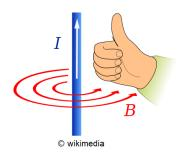
As charges flow through a wire, magnetic field lines will form concentric circles perpendicular to the direction the current moves.
