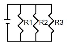
In a parallel series, a wire will connect to multiple resistors, each of which will end at the same point. Charges will only pass through a single resistor in a parallel circuit.
