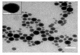
Transmission electron micrograph of silver nanoparticles
