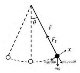
Choosing the instantaneous Cartesian co-ordinate system as shown in the figure, and separating the force mg into its components along those axes, we can write the following according to Newton's second law of motion:
