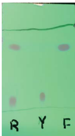
Figure 3. TLC plate showing red crystals (R), yellow crystals (Y), and fluorenone starting material (F)
