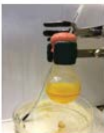
FIG. 2 SYNTHESIS 2: REACTION IN GLYCEROL BATH
